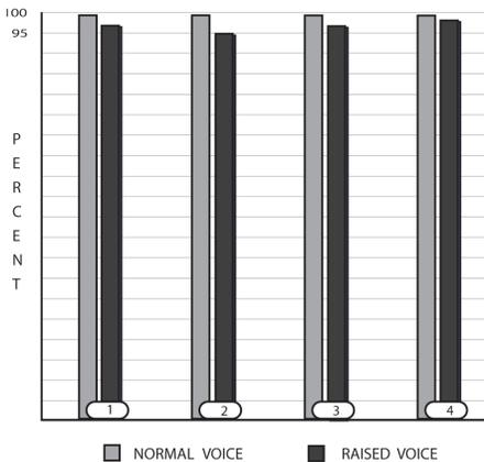
Figure 1 illustrates the Privacy Index achieved in the lab for 3 types of wall panels, one ceiling and on both carpeted and vinyl floors.
